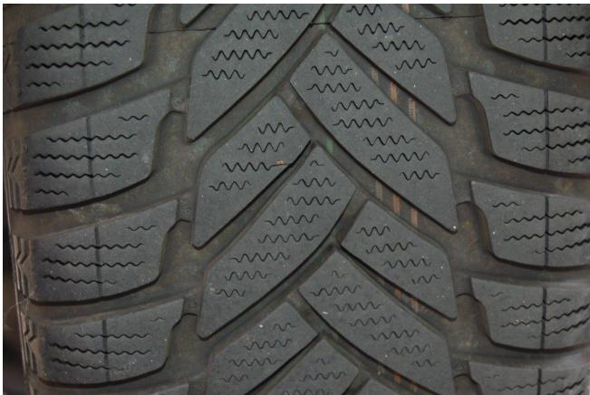
KUMHO Solus 205x65x16 on the Valkyrie - new tire with only about 1k on it so far - no mods required to fit this tire.
