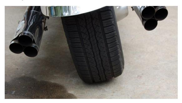
Bridgestone Battlax BT45r front tire used on both bikes - the r stands for rear not radial. This is fairly common on the Bias tires, the mark them as front or rear but normally the rear tires work better on big bike rims. There is no difference in the construction or design.
