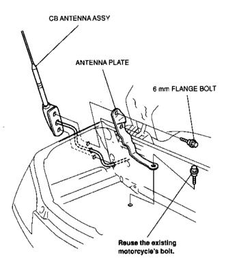
Route and connect the antenna harness to the CB antenna harness, then reinstall the left pocket.
