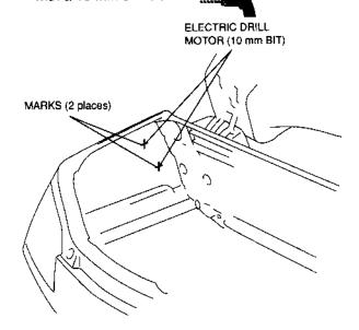
Locate the mark on the outside of the motorcycle trunk and drill a hole through the mark using an electric drill motor starting with a 3 mm, 6 mm, and finally with a 13 mm drill bit.
