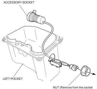
NUT (Remove from the socket before routing the harness through the 30 mm hole in the pocket.)
