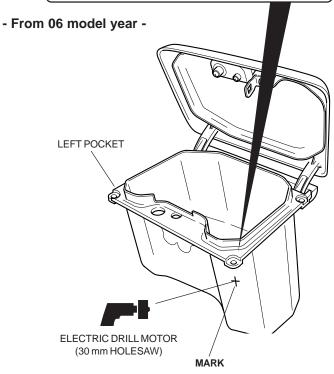
4. From the inside, route the accessory socket harness connector out through the 30 mm hole, then install the socket in the 30 mm hole. Secure the socket with the nut as shown.
