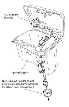
5. Connect the accessory socket harness connector to the motorcycle's harness connector. Pull the connector cover over the connectors.
